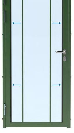
Fit beading screws into predrilled holes to perimeter of aperture (this must be done after glass is in position to avoid damaging glazed units).
